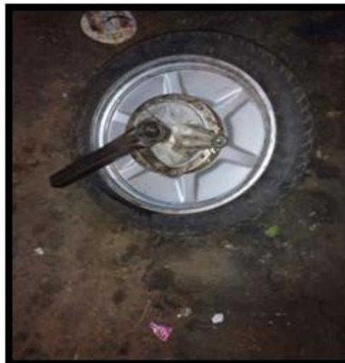
Figure: Drum Brake
