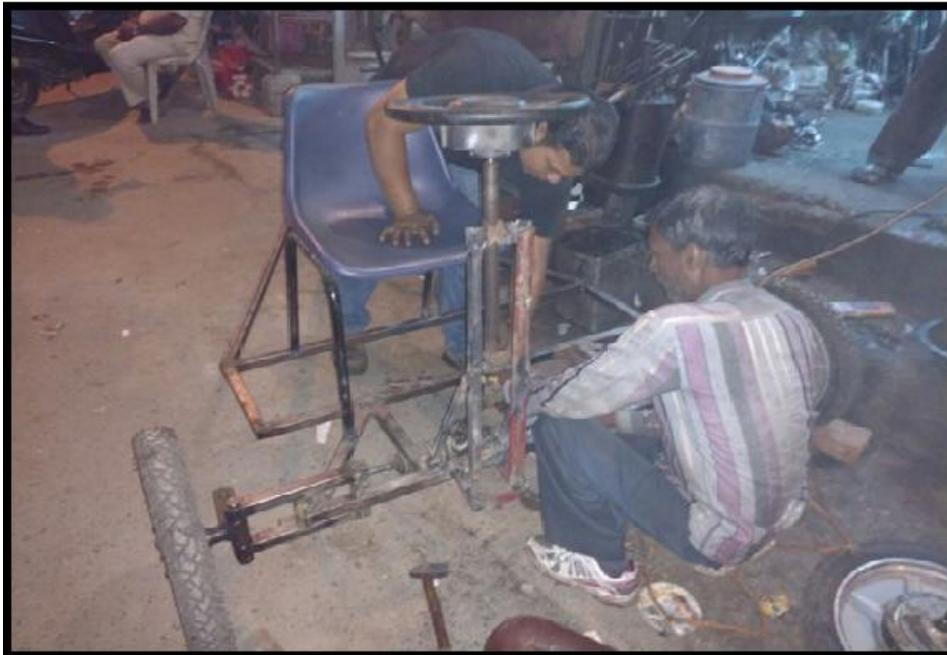
Figure: Workers helping in Adjusting Steering Column.
